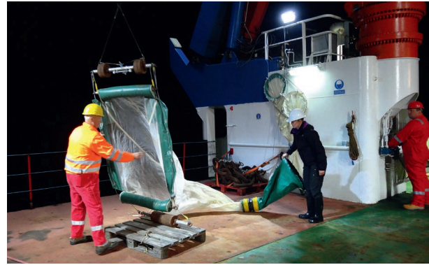
Fig. 8. Preparing the Rectangular Midwater Trawl (RMTFF) for sampling of zooplankton during Atlantic Meridional Transect 22 in 2012.
